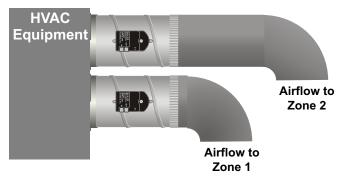
Ensure that damper installation does not cause obstruction to the damper blade.
